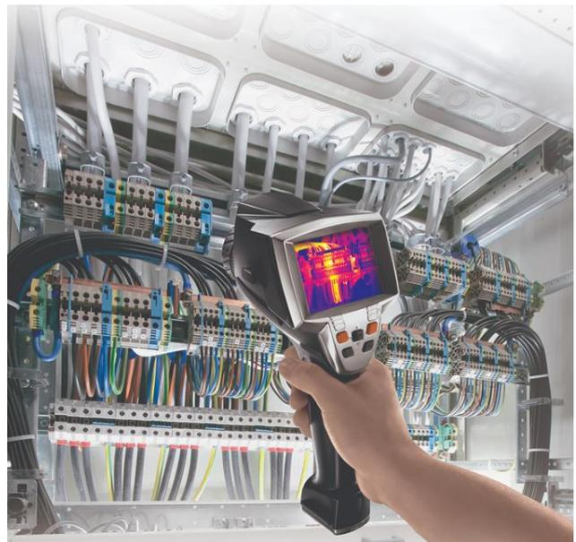
Thermal imaging cameras will precisely locate and record hot spots or heat sources, often deeply buried in the electrical circuits, which can very quickly lead to electrical fires.
